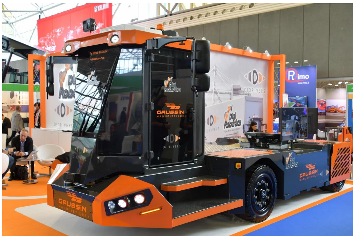
Photo of APM « Autonomous Prime Mover »- The world's first autonomous electric truck
